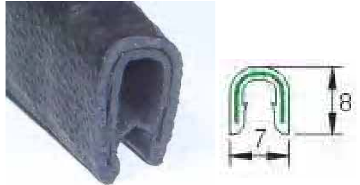
MINI EDGE TRIM #TRMPS Patterned PVC with steel reinforcing. Max panel thickness 2.5mm. Channel depth 7mm. Will form to 30mm radius curves. £2.50/mtr (£2.93 inc vat)
